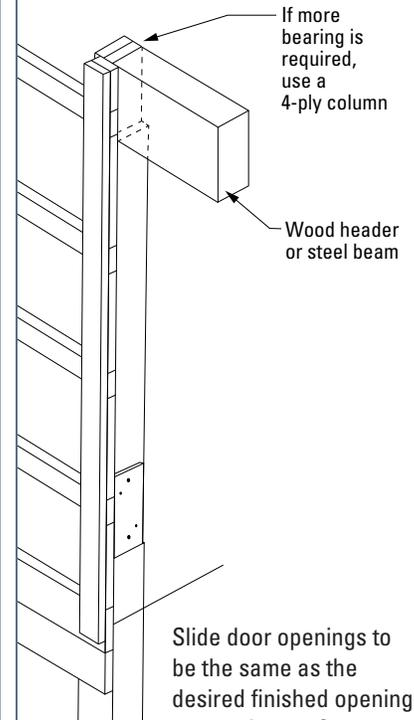
Slide door openings to be the same as the desired finished opening. Perma-Column® brackets intrude into the slide door opening by 3/8".
