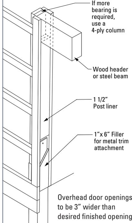
Overhead door openings to be 3" wider than desired finished opening to accommodate 1 1/2" Perma-Column® bracket trim-out.
