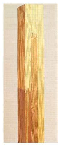
**Assembly (finger joint):** For longer length columns separate lengths of wood are joined together with a glued finger-jointing process.
